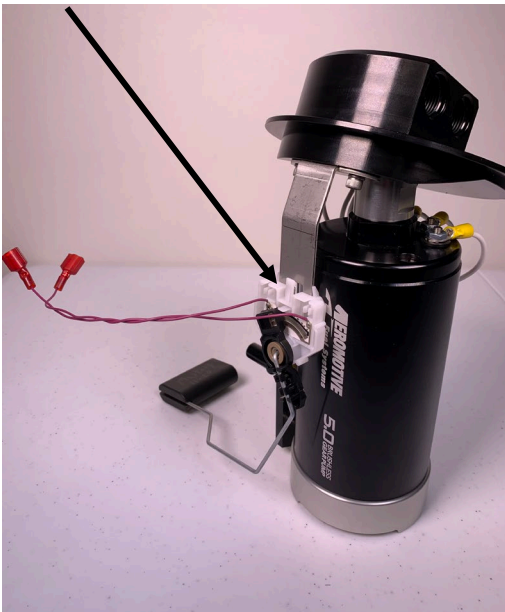
Fuel Level Sensor properly installed on bracket.
