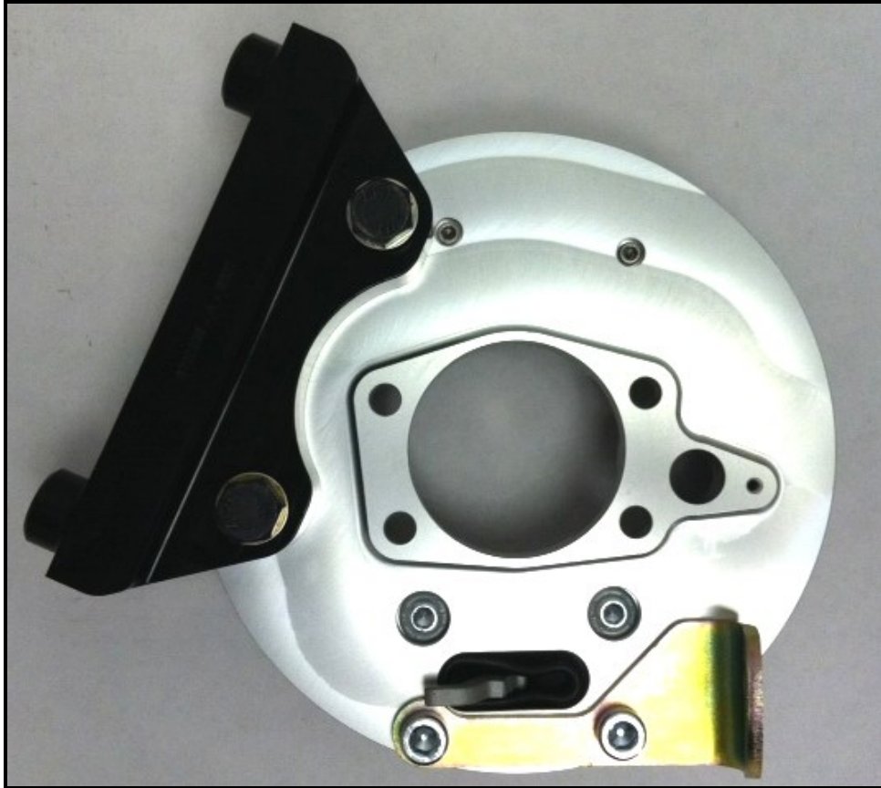
Figure 3: Park brake assembly correctly installed (driver's side)
