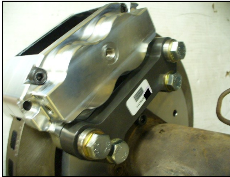
Figure 5: Caliper installed on intermediate bracket
