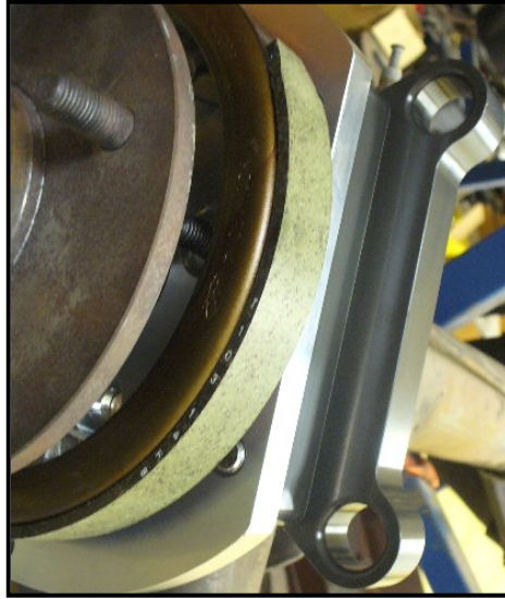
Figure 3: Park brake assembly correctly installed
