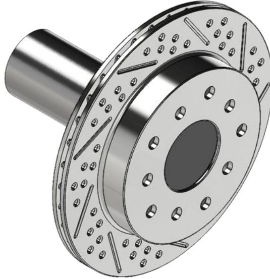
7. Install the correct side rotor, referring to the "Rotor Installation and Rotation" instruction included in the promotional packet provided with this system. Ensure the inside of the rotor hat sits flush against the mounting face of the axle flange to prevent excessive rotor runout.
