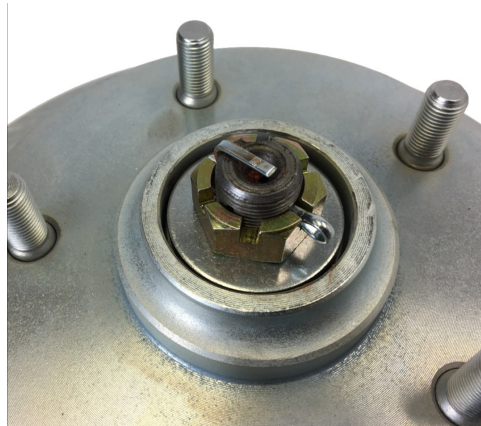
Figure 6. Cotter pin installed
