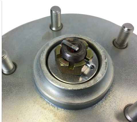
Figure 5. Cotter pin installed (classic spindle nut shown in photo, 1970+ systems included spindle nut and retainer)
