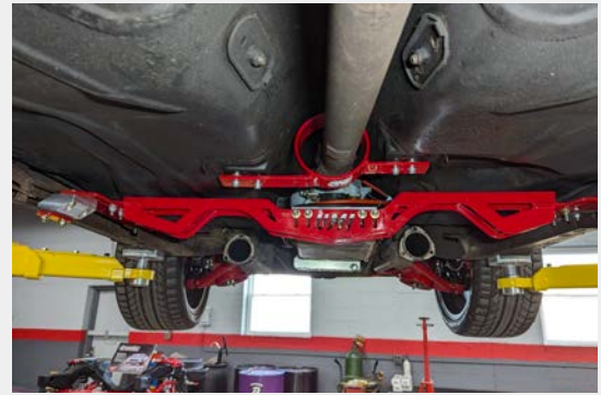
Figure 1: Fully Installed Crossmember
