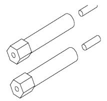
8. Locate the two 7/16" mounting holes on the block, looking at the front of the engine block there will be two 7/16" threaded holes oriented vertically from each other to the right of the crankshaft. Thread each of the spacer / stud assemblies into each of the two mounting holes and tighten.
