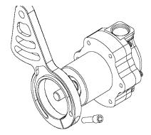
11. Using the two 3/8-16 X 1" bolts and two 3/8" flat washers attach the fuel pump bracket to the spacers; leave the assembly loose until final alignment can be determined.
