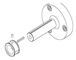
7. Thread each of the  $7/16-14 \times 1\frac{1}{2}$  studs into each of the two spacers
