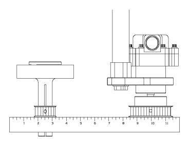
16. Once the pulleys are aligned, tighten the pump bracket screw and both pulley setscrews. It is recommended to use a removable Loc-tite thread locker on the setscrews to prevent them from loosening during operation.
