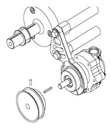
15. Using a straightedge align the pulley on the crankshaft with the pulley on the fuel pump. Alignment may be achieved by moving the pump location in the mounting bracket and by moving the location of the 14-tooth pulley on the drive mandrel. In some cases it may be necessary to shorten the pump bracket spacers to accommodate other accessories on the drive mandrel.
