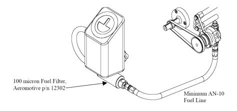
21. Connect the fuel pump outlet to the fuel filter inlet. We recommend using fuel filter Aeromotive p/n 12301, utilizing a minimum of AN-08 steel braided fuel line. Next, connect the fuel filter outlet to the vehicle's fuel system. **Make sure you use high pressure (1000 psi minimum) fuel line for these connections!**
