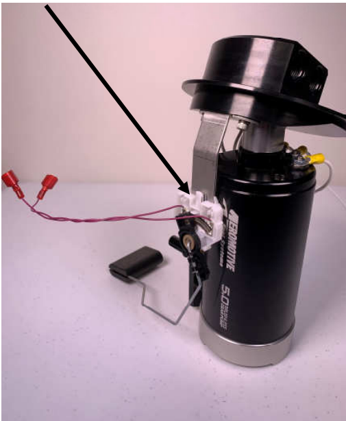
Fuel Level Sensor properly installed on bracket.
