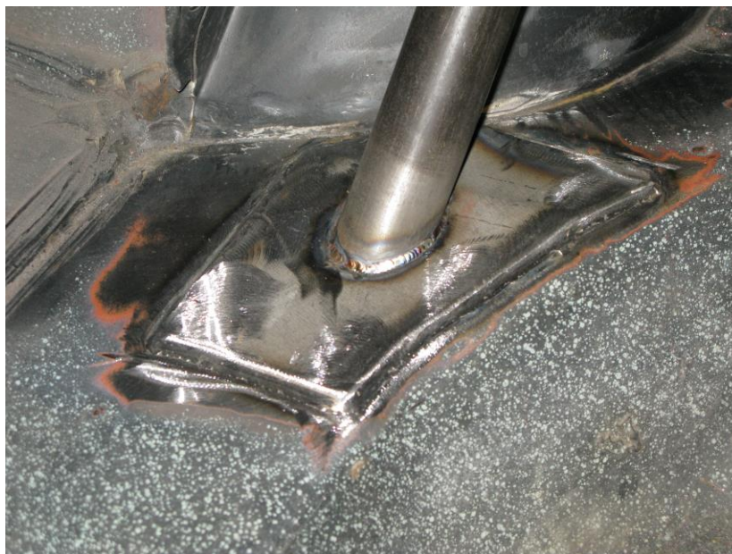
Figure 1 – Trunk Doubler Installed
