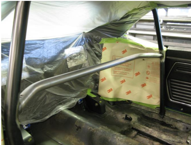
Figure 12 – Finish Weld Cross Brace
