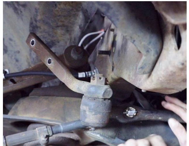
Figure 6 - Remove Idler Arm
