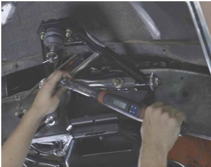
Figure 47 – Torque Upper Control Arms
