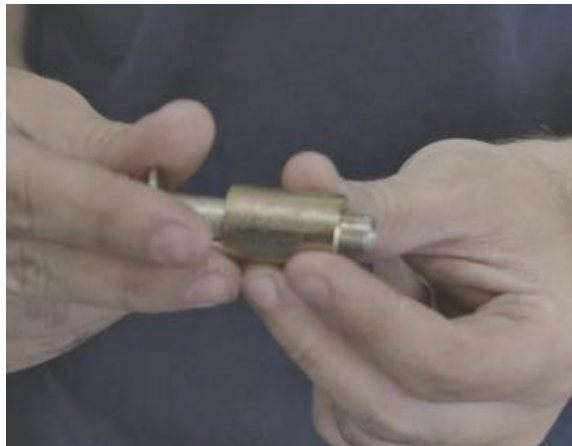
Figure 83 – Place Crush Sleeve Over Lower Shock Bolt
