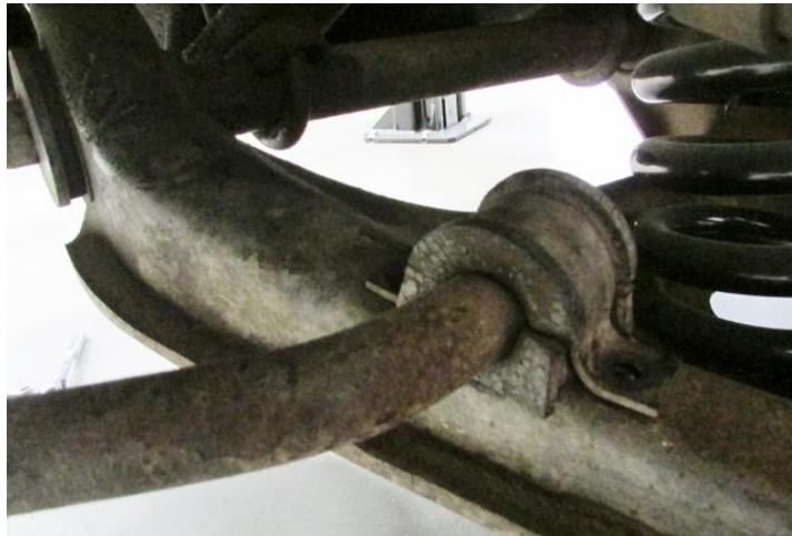
Figure 2 - Remove Sway Bar
