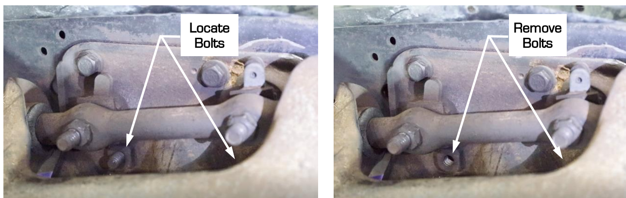
Figure 15 - Remove Lower Upper Control Arm Bracket Bolts
