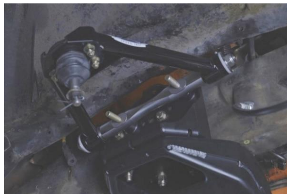
Figure 45 - Install Upper Control Arms
