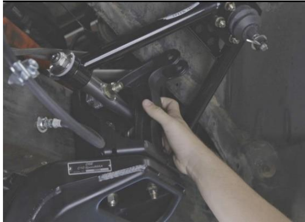
Figure 48 - Position Upper Coilover Mount
