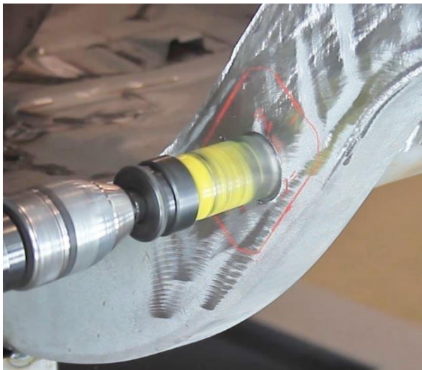
Figure 9 – Drill Upper Link Hole & Tack Weld Doubler Plate
