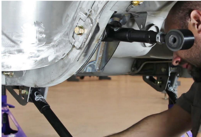
Figure 39 – Install Upper & Lower Links
