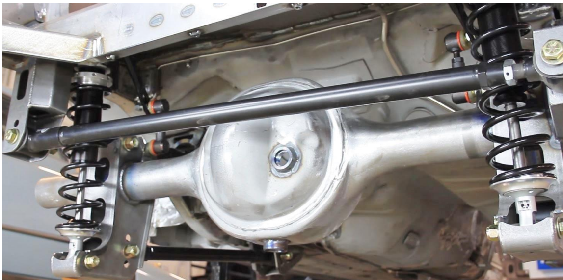
Figure 49 – Install Track Bar
