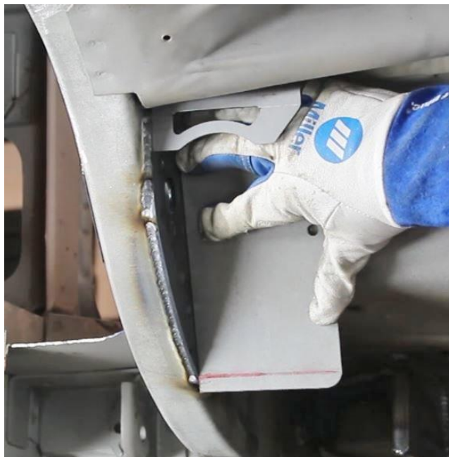
Figure 13 – Trim Front Upper Link Mounting Bracket
