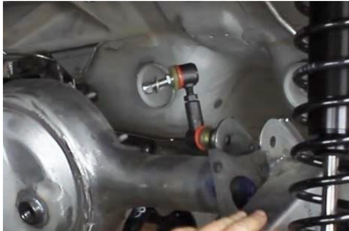
Figure 45 – Install Sway Bar End-Links onto Axle Brackets
