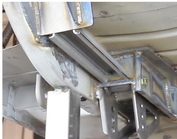
Figure 21 – Fit Upper Link Mount Braces
