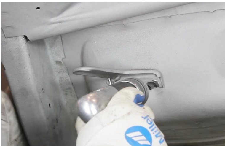
Figure 6 – Remove Brake Line Bracket
