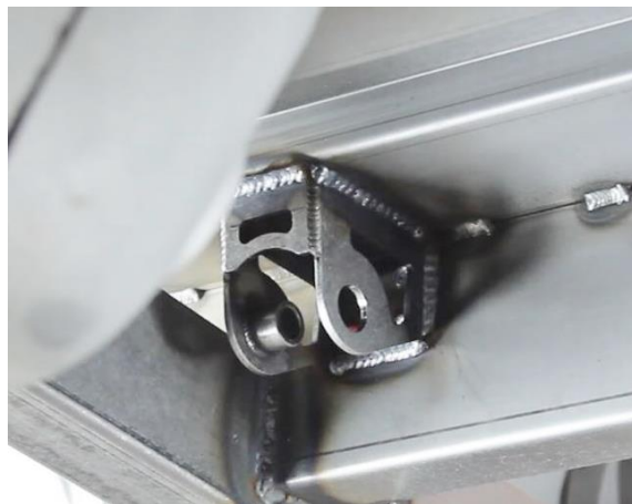
Figure 26 – Weld Upper Shock Mounts
