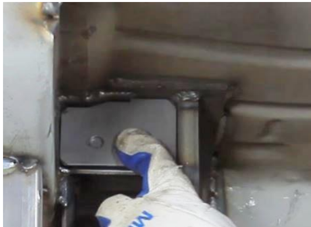
Figure 20 – Locate Lower Link Closeout
