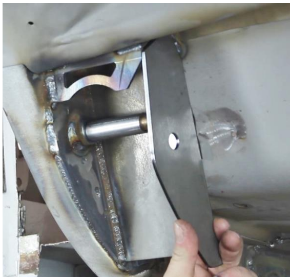
Figure 16 – Locate Inner Upper Link Mount Closeout
