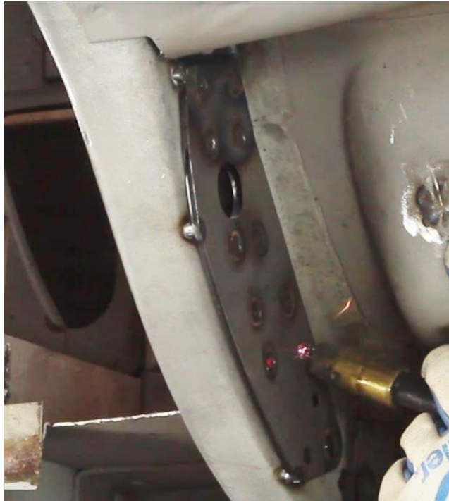
Figure 12 – Weld Outer Closeout Bracket
