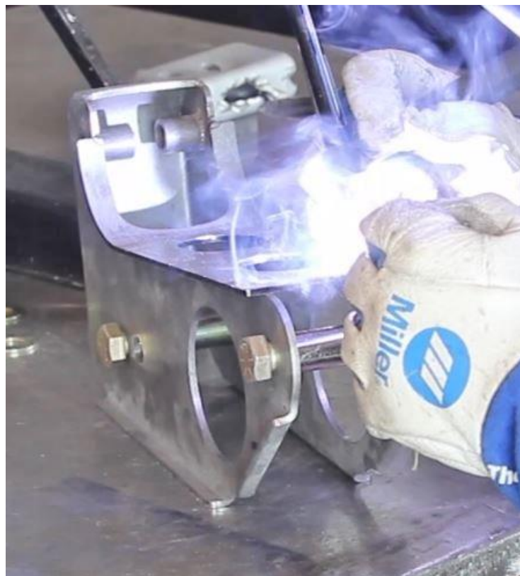
Figure 32 – Weld Axle Bracket Reinforcement
