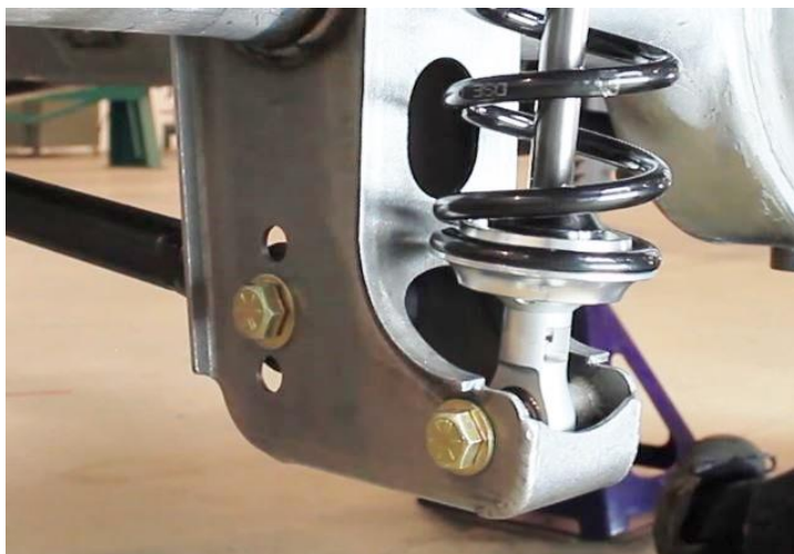
Figure 47 – Install Coilover Shocks
