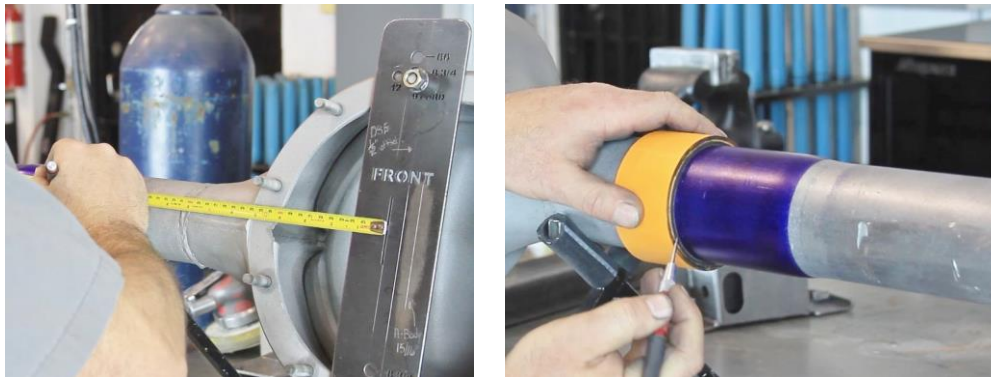
Figure 34 – Locate Axle Brackets on Axle Tubes
