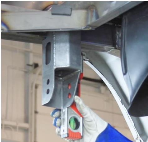
Figure 30 – Weld Track Bar Body Bracket
