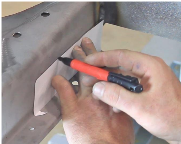
Figure 27 – Cut Out Front Trunk Corners
