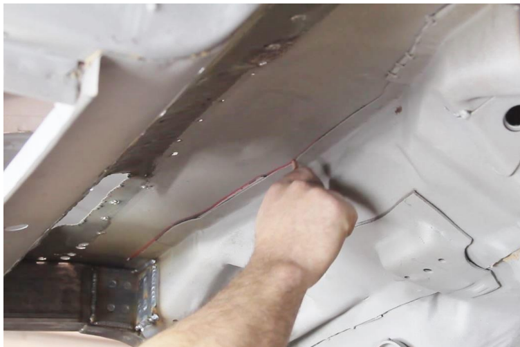
Figure 1 – Mark Floor Pan Cut Line (Underneath Vehicle)
