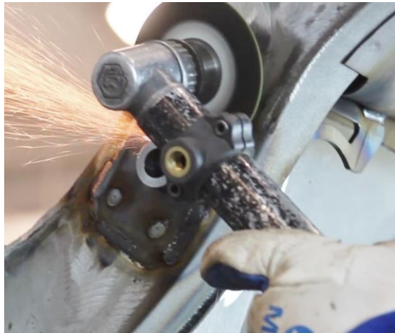
Figure 15 – Cut-Off Crush Tube Flush with Frameraill
