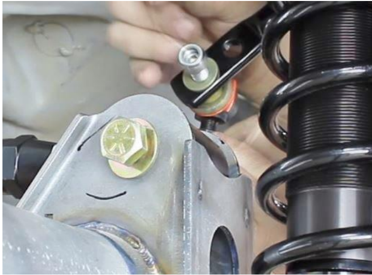
Figure 48 – Attach Sway Bar End-Links
