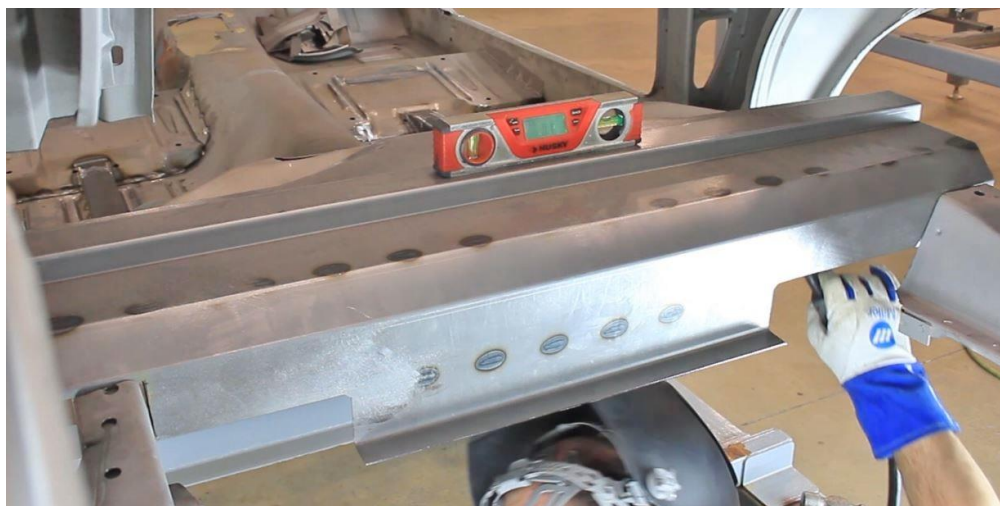
Figure 23 – Weld Upper Crossmember
