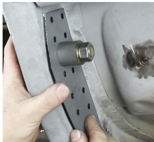
Figure 11 – Locate Outer Closeout Bracket
