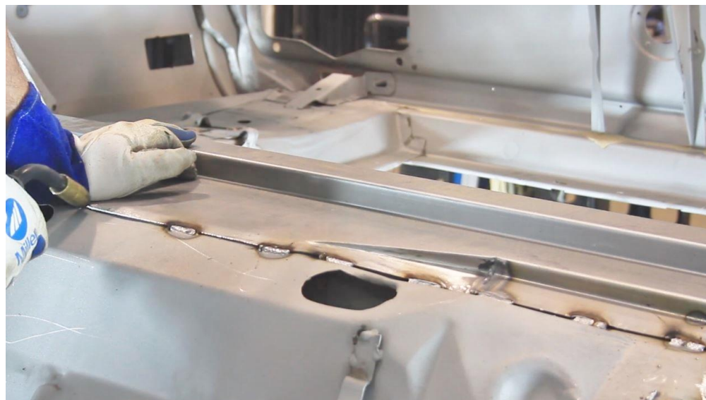
Figure 24 – Stitch Weld Front of Crossmember
