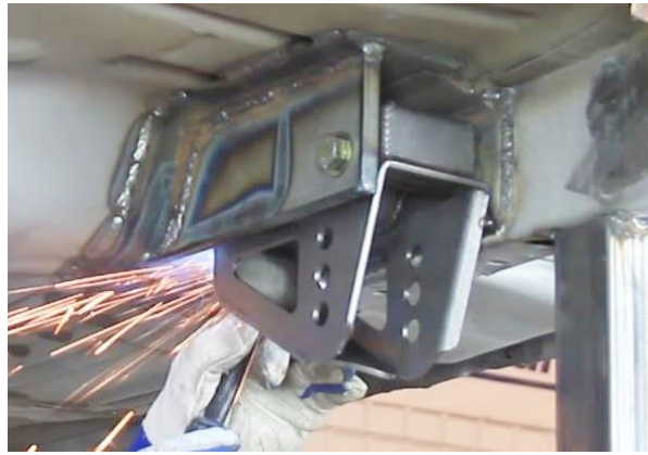
Figure 19 – Weld Front Lower Link Bracket
