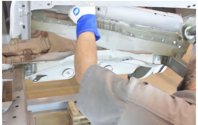
Figure 5 – Remove Trunk Floor Section
