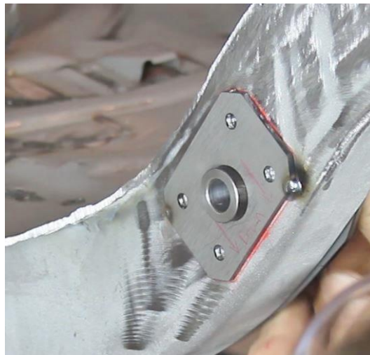
Figure 10 – Install Outer Closeout Bracket & Crush Tube
