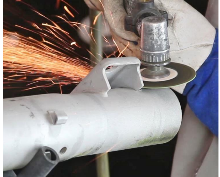
Figure 31 – Remove Housing Ends & Leaf Spring Brackets
