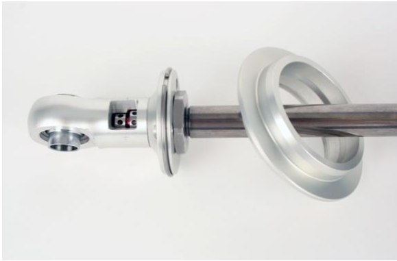
Figure 41 – Removing the Upper Spring Seat
