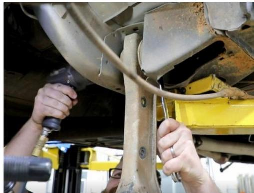
Figure 8 - Remove Factory Lower Link
