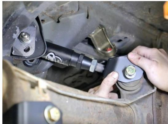
Figure 7 - Install Upper Swivel-Link™
