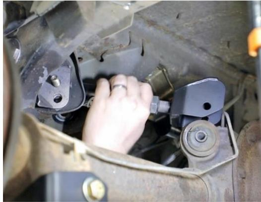
Figure 6 - Install Upper Swivel-Link™
