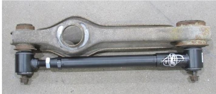
Figure 9 – Detroit Speed vs. Stock Lower Link
