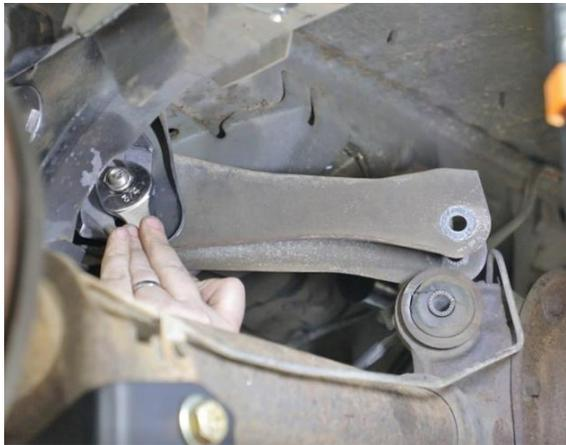
Figure 4 – Remove Factory Upper Link
