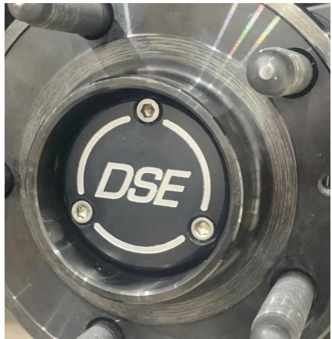
Figure 20 – Install Detroit Speed Hub Cap
