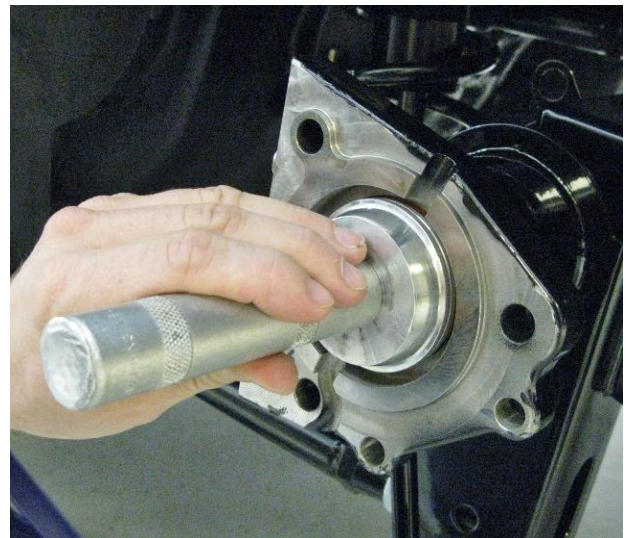
Figure 3 - Install Axle Seals
