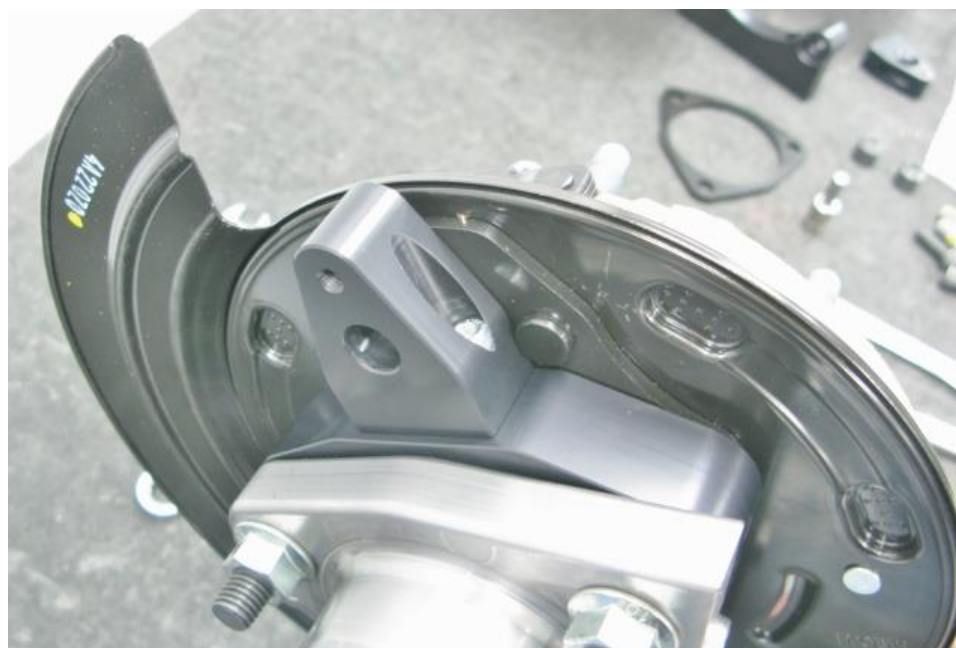
Figure 7 – Install Park Brake Mount
