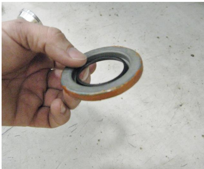
Figure 2 - Use RTV on the Axle Seals
