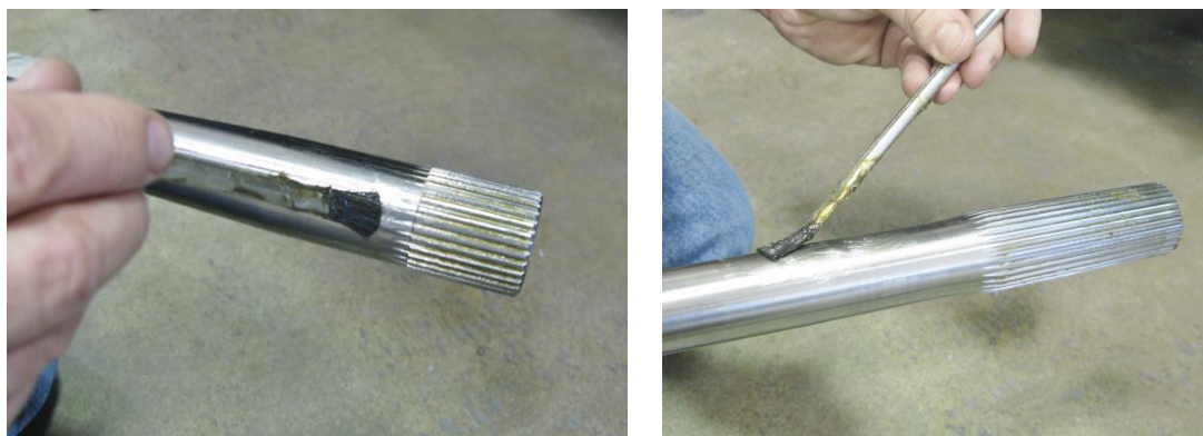
Figure 16 – Grease Axle Shafts
