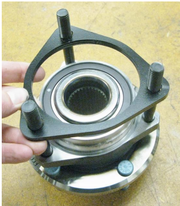
Figure 8 – Install Hub Shim
