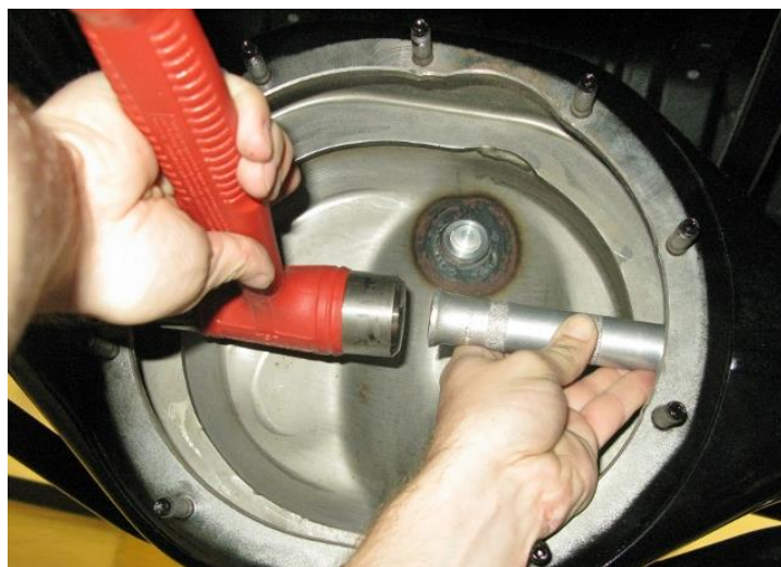
Figure 15 – Install Inner Axle Seals
