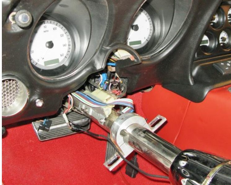
Figure 22 – Remove Steering Column
