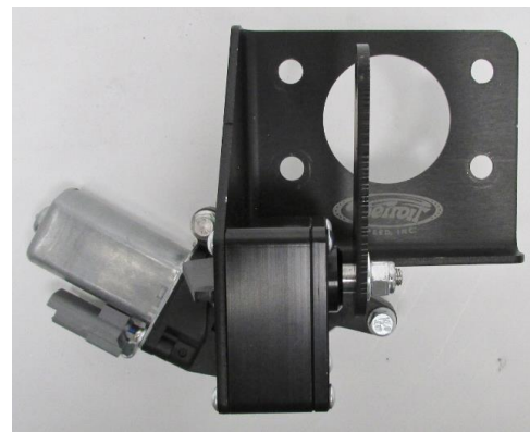
Figure 10 – RH or Passenger Side Actuator
