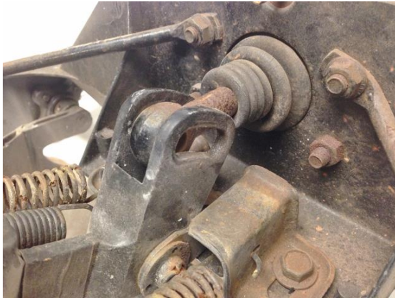
Figure 3 – Remove the Pivot Pin
