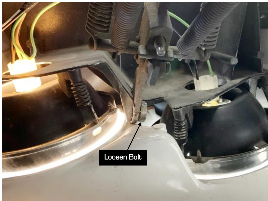
Figure 38 – Loosen Headlight Door Bolt
