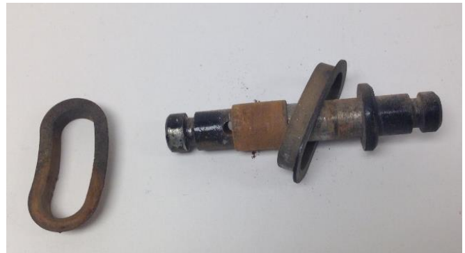
Figure 4 – Pivot Pin & Bushings
