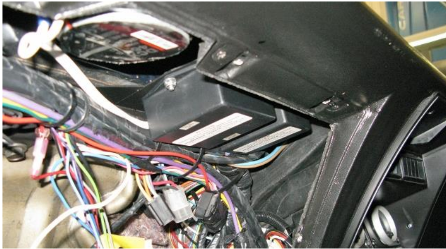
Figure 35 – Mount Headlight Module (Wiper Module also Shown)
