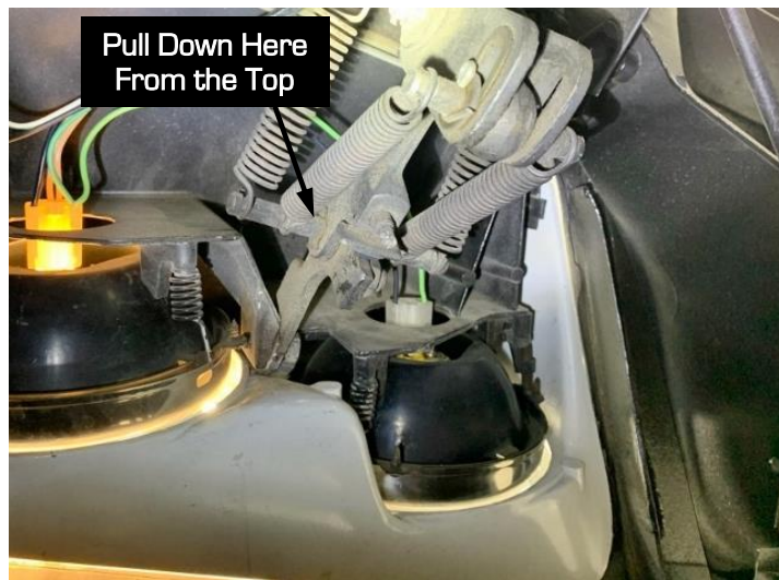
Figure 8 – Manually Close Headlight Door
