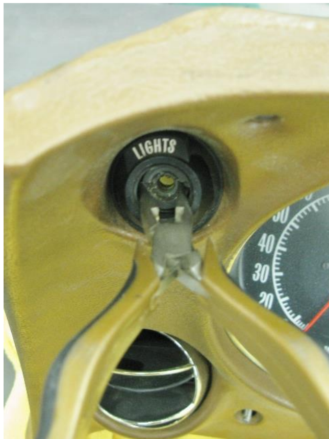
Figure 25 – Remove Retaining Nut
