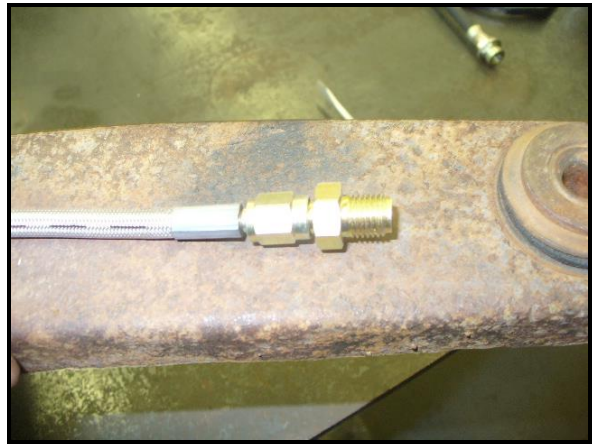
Figure 6: Install adaptor into AN fitting on hose
