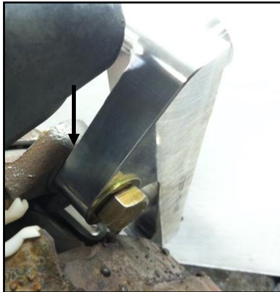
Figure 4: Shim location is between both brackets
