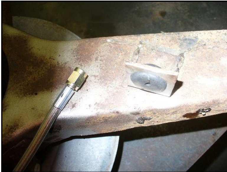
Figure 1: Supplied rubber grommet installed in swing arm bracket
