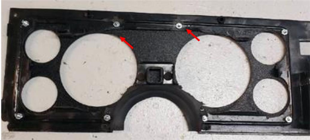
Remove the nuts and lock washers from the studs on the back of the panel.
