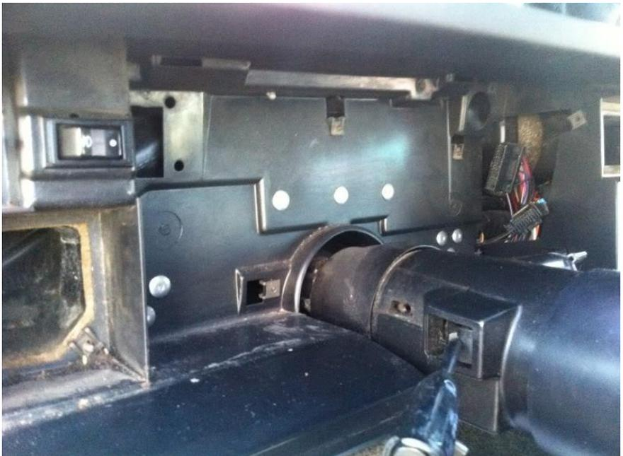
Prepare to install the adapter bracket. This will do directly over the front of the dash panel and attach directly to that panel
