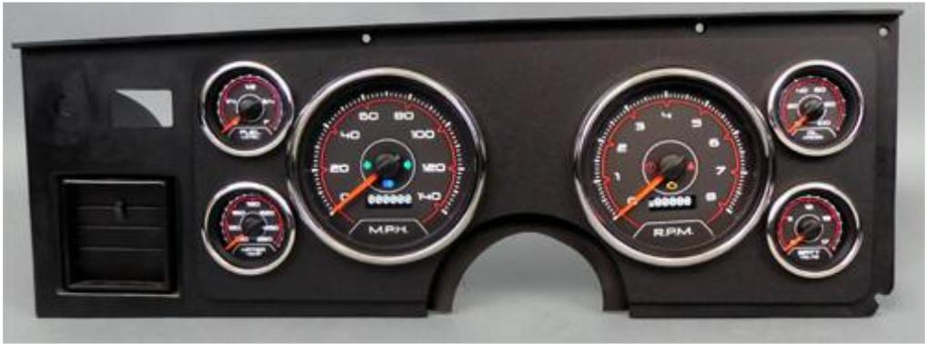
Gauge wiring should follow the gauge booklet. Splice into the factory harness at the plug. You may opt to leave the OE plugs in place and splice in behind it (recommended) retaining the factory plugs. Just tape off the plug when completed wiring. Use the 6-gauge kit diagrams on 23-24 in your book.
