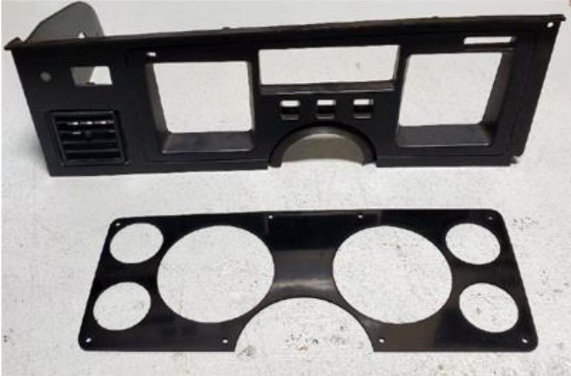
Line up your template to cover the detail line on the panel around the factory gauges. Do not cover the panel fasteners (red arrows), stay just below them. Attach with tape to hold secure.
