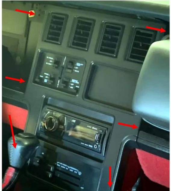
Remove the 4 socket head screws shown below. Once those are removed the part can be tilted back and then out. Remove the plugs from the cluster. BYE!
