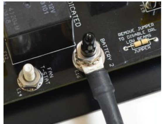
Detail of Daytime Running Light (DRL) Jumper and Proper Power Lead Connection
