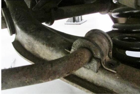
Figure 1 - Disconnect Sway Bar
