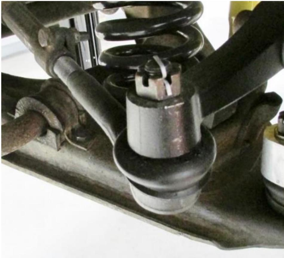
Figure 10 – Install Outer Tie Rod
