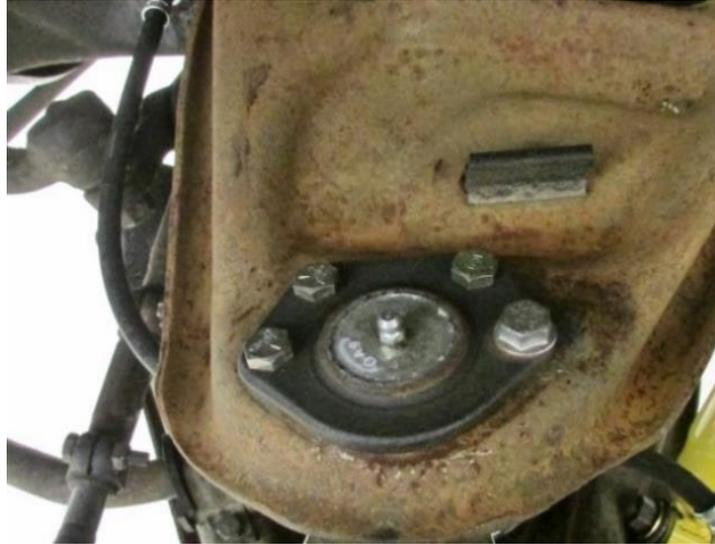
Figure 5 – Replace Upper Ball Joint
