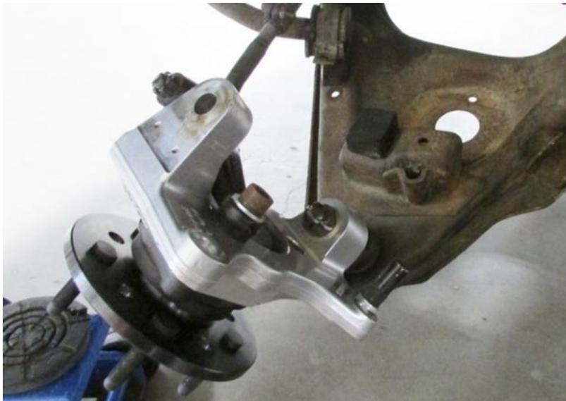
Figure 6 – Install Upright Assembly
