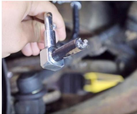
Figure 2 - Remove Brake Hose
