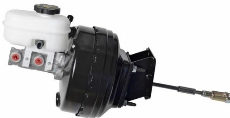
Figure 12 - Brake Booster/Master Cylinder Kit
