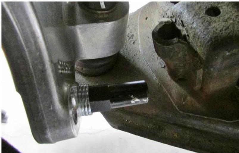
Figure 15 – Steer Stop Adjustment
