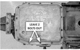
**17. Install the pan and new gasket** using 12 of the 14 the original bolts. (Do not tighten yet.) Leave out the 2 bolts behind the selector lever for the cable bracket.
