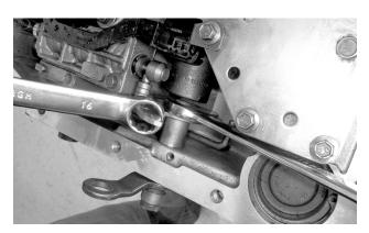
Loosen the selector shaft nut with a 21mm wrench, and a smaller box wrench hooked over the inner selector lever.
