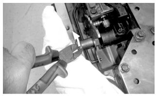
5. Protect the case flange with a rag, and use diagonal cutters to remove the selector shaft retaining pin from the case.
