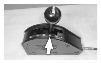
A. With the selector lever still in OD (from Step 20) and the shifter in DRIVE (or 3), adjust the cable bracket nuts (and swivel, if necessary) until the swivel slips freely in and out of the selector lever hole.
