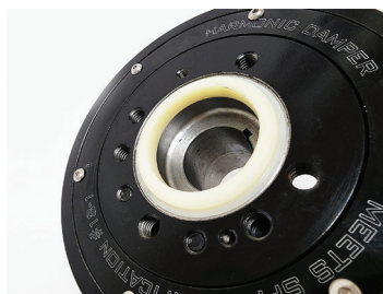
Nylon Ring for 4-bolt applications
