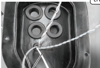
Route heavy gauge orange and white wires through 7/8" wiring grommet on kick panel
