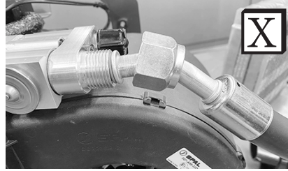
Improperly Seated O-ring Land
