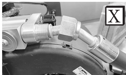
Improperly Seated O-ring Land
