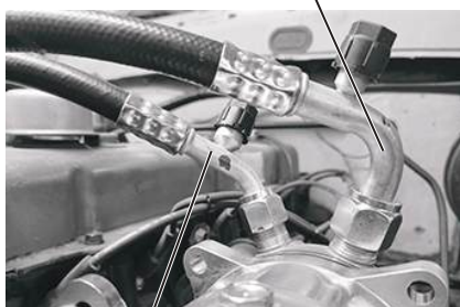
Connect #8 45° fitting with service port to #8 discharge port on compressor
