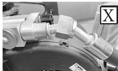
Improperly Seated O-ring Land
