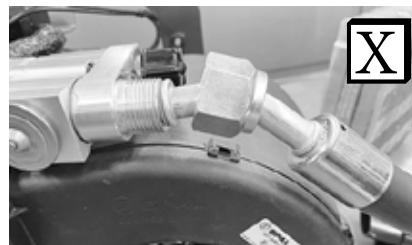
Improperly Seated O-ring Land
