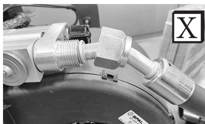
Improperly Seated O-ring Land
