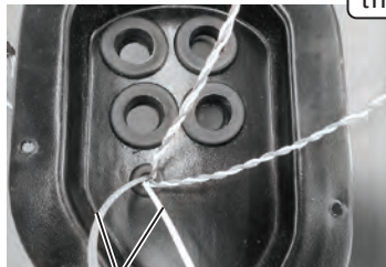
Route heavy gauge orange and white wires through 7/8" wiring grommet on kick panel cover
