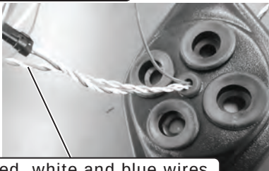
Route red, white and blue wires from main harness through 7/8" wiring grommet on fresh air cap
