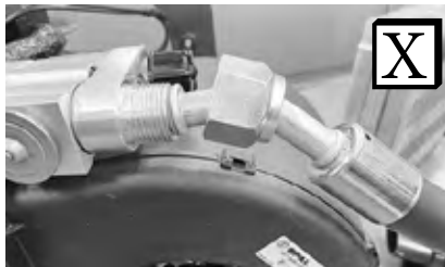
Improperly Seated O-ring Land
