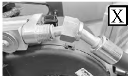
Improperly Seated O-ring Land
