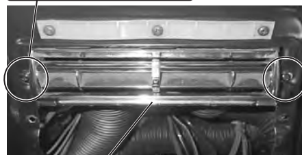
Install center louver assembly into dash
