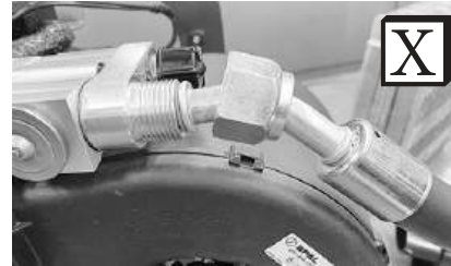
Improperly Seated O-ring Land
