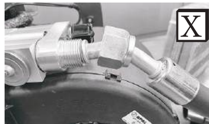
Improperly Seated O-ring Land
