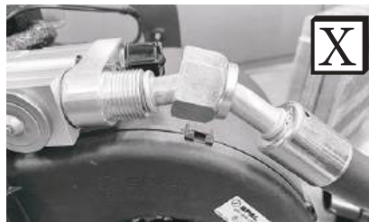
Improperly Seated O-ring Land
