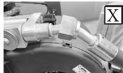
Improperly Seated O-ring Land
