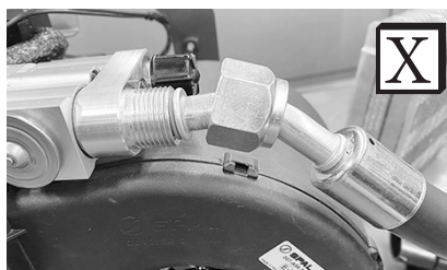
Improperly Seated O-ring Land
