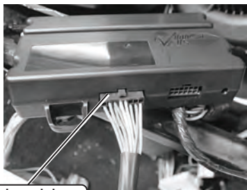
Plug main wiring harness into ECU
