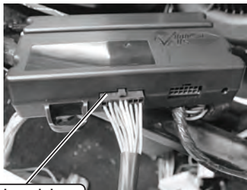
Plug main wiring harness into ECU
