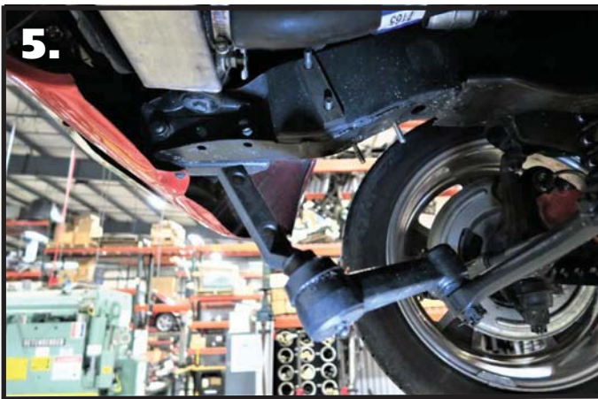
5. Disconnect the idler arms from the frame.
