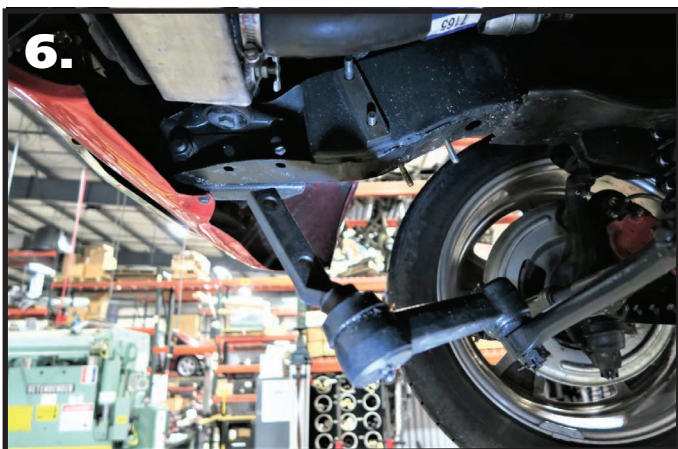
6. Disconnect the idler arms from the frame.
