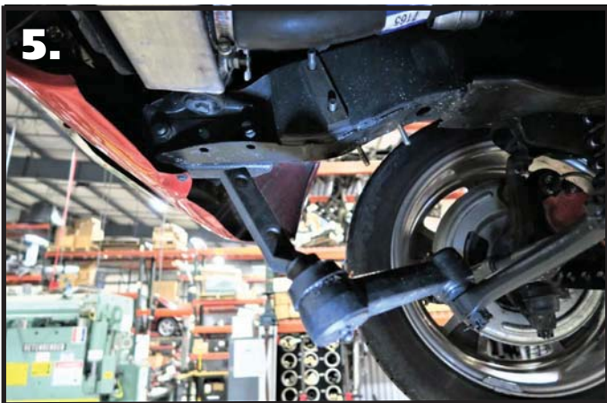
5. Disconnect the idler arms from the frame.
