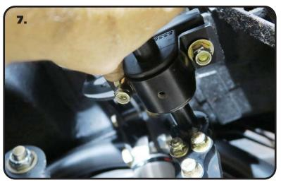
7. Insert the MuscleBar up into the car with the Arms pointing forward. Line up the holes in the Bushing Straps with the Bolts sticking down out of the mounts on the crossmember. While holding the bar in place, install a 3/8" Flat Washer and 3/8"-16 Nylok Nut on each of the (4) bolts sticking through the bushing straps. Torque the hardware to 45 ftlbs.
