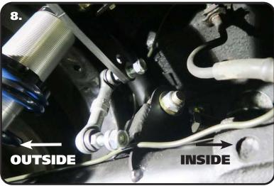
**8.** Install a 3/8" Flat Washer on the threads of one end of the PosiLinks. Insert the PosiLink into the OUTER hole of the musclebar arm with the threads pointing to the inside of the car. Refer to **Image 8**. Install a 2nd 3/8" Flat Washer on the inside of the arm followed by a M10-1.5 Nylok Nut. Repeat on the other arm with the threads pointing to the inside of the car. Torque the Nuts to 37 ftlbs.
