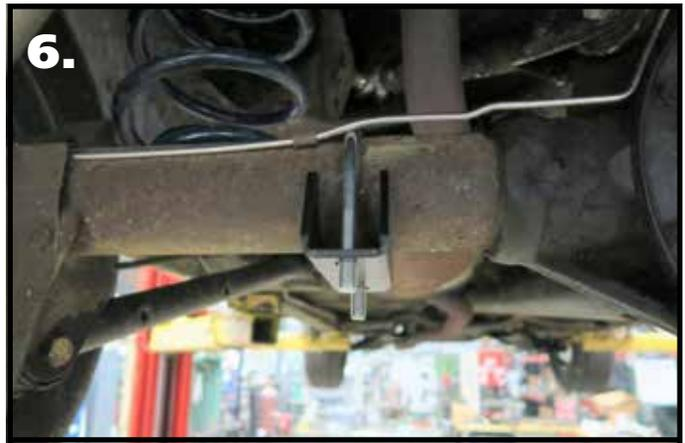
**6.** Install an axle bracket onto each u-bolt with the flat side to toward the ground. The "teeth" of the mount should touch the axle tube.
