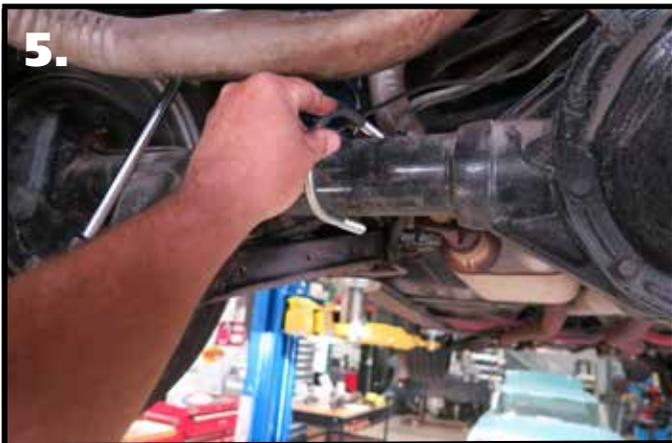
**5.** Install the u-bolts onto the axle tube with the threads pointing down. You may need to raise the brake lines in the area of the u-bolts. The u-bolts will be approximately 23 1/2" apart and equal distance on each side from the brake backing plates.
