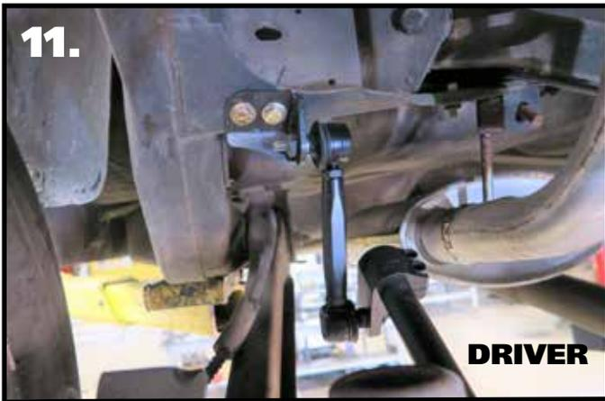
**11.** Swing the tab up to the frame, keeping the linkage straight from side to side. Use the tab to mark the location of the holes that will need to be drilled. Drill the holes with a 3/8" drill bit. Install a 3/8" flat washer on each of (2) 3/8"-16 x 1 1/4" hex bolts and install them through the bracket and drilled holes. Install a 3/8" flat washer & 3/8"-16 nylok nut on each bolts sticking through the frame. Torque the hardware and repeat on the other side.
