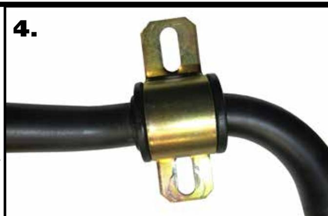
**4.** Install the bushing straps over the sway bar bushings.
