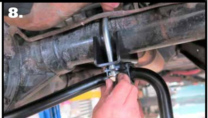
**8.** Hold the sway bar in position on the car with the center bend toward the ground. Install a 7/16" flat washer & 7/16"-20 nylok nut on the threads of the u-bolts. Snug the hardware down and verify that it is centered and the axle mounts are level. Torque the u-bolt hardware.
