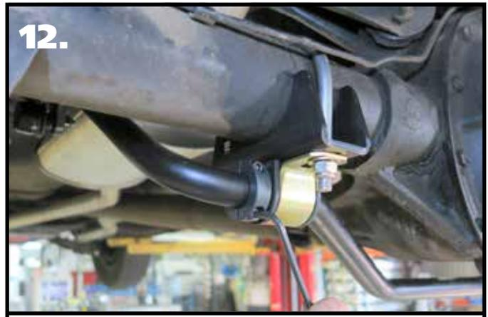
**12.** Install the locking rings on the outside of each bushing assembly. Use a hex key to take the locking ring apart. Reassemble it on the bar positioned next to the outside of the bushing assembly. Push the locking ring up against the bushing assembly and tighten.
