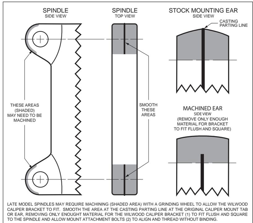
Figure 3. Machining Diagram
