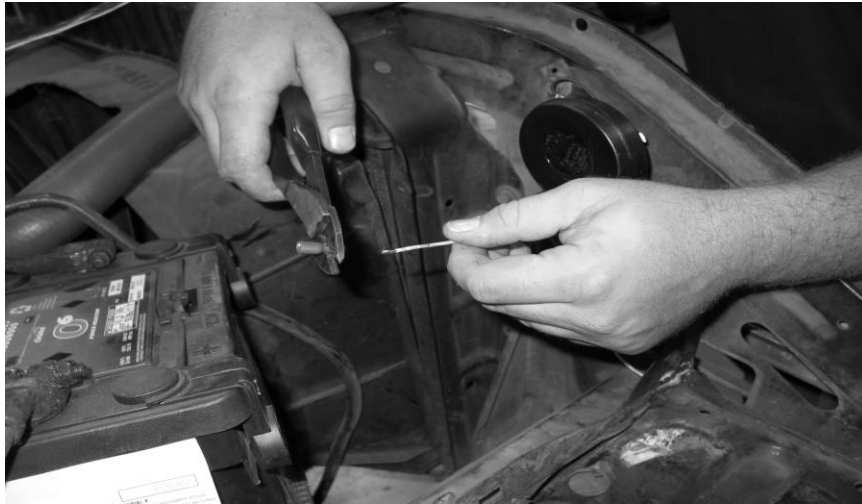
Figure 7-4 Horn Connections (All Models)
