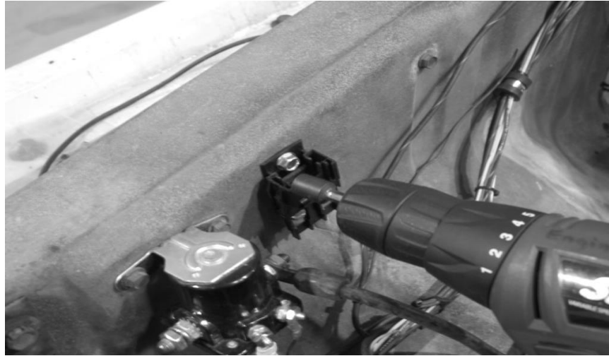
Figure 7-6 Installing the Maxi Fuse Holder '73-'77 Model
