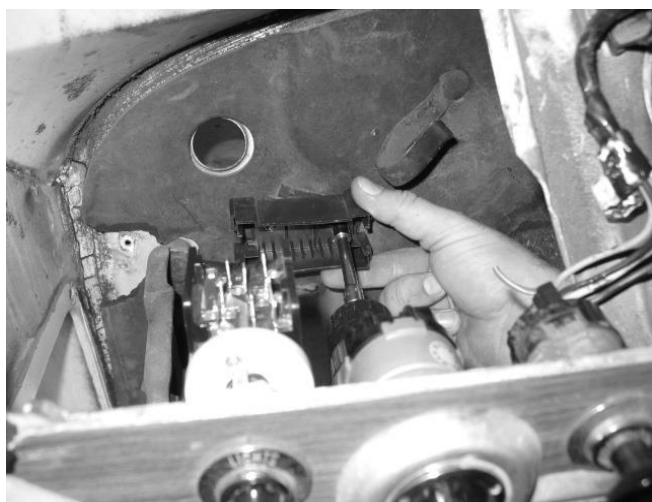
Figure 6-2 Fuse Block Base Position '67-'72
