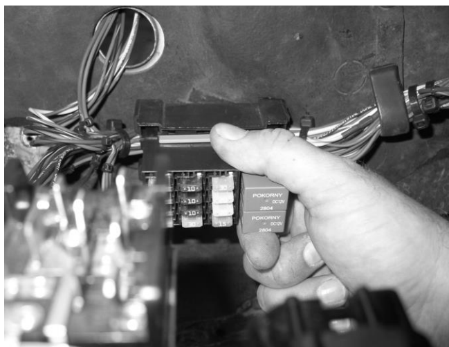
Figure 6-5 Snapping Fuse Block into Base
