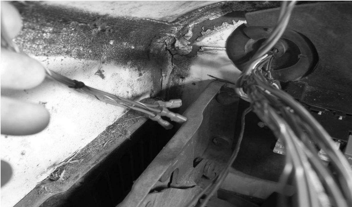
Figure 7-22 Routing the Dimmer Switch Wires
