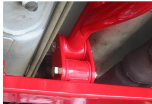
**Figure 2:** Torque Arm Attached using Pivot Plates
