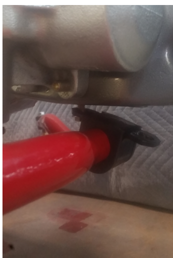
Figure 1) Front bolt removed and rear bolt loosened
