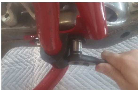
Figure 3) Tighten sway bar bolts down once all four bolts are started
