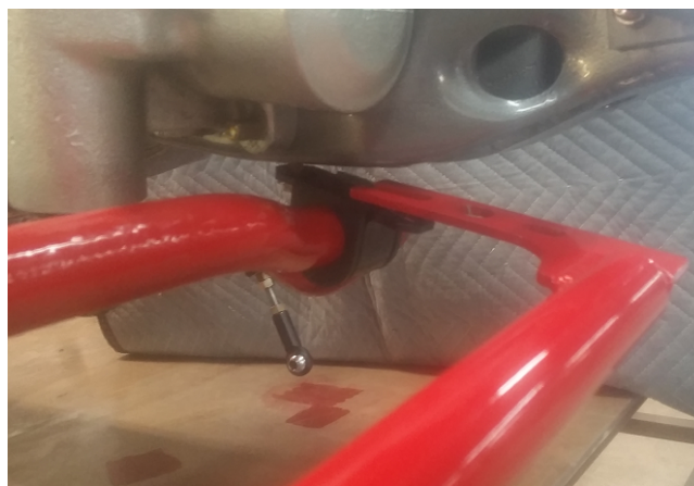
Figure 2) Inserting brace slots onto the rear sway bar bolt
