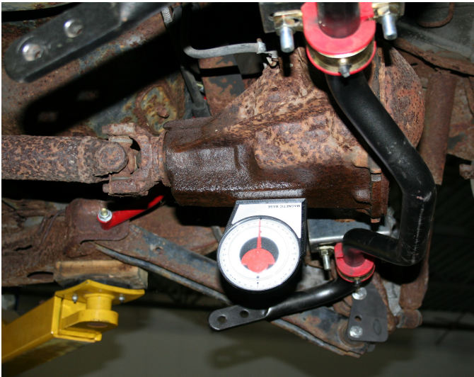
IMAGE #1: (Measure & Record Yoke Angle)
