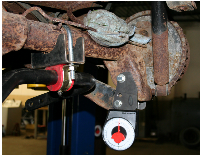
IMAGE #2: (Match Bracket Angle To Yoke Angle)
