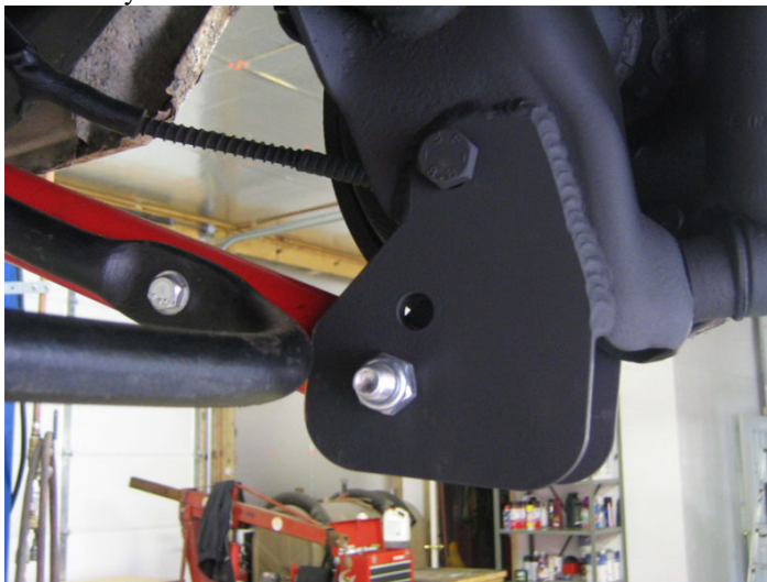
Image 4- Passenger lift bar bracket installed with control arm and sway bar.
