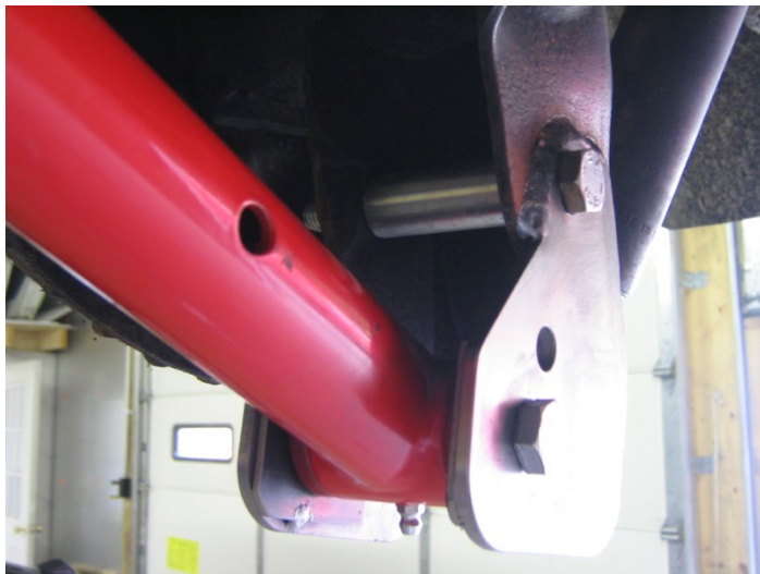
Image 1- Drivers side brackets installed and welded
