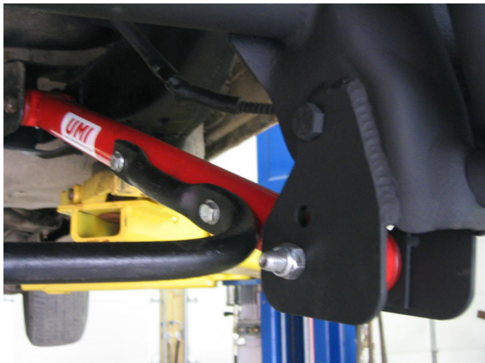
Image 3- Shows installation of lift brackets completed.
