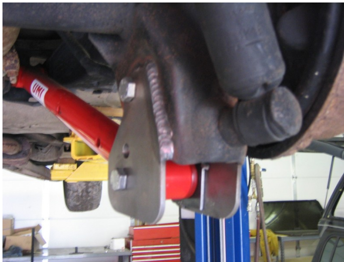
Image 2- Passenger Side installed and welded
